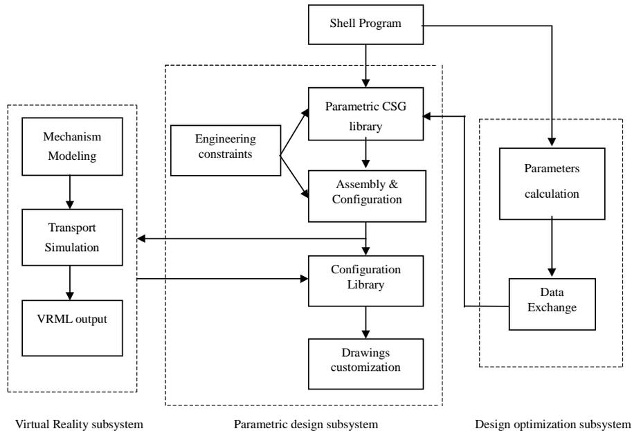
Fig.1 Structure of design automation of blending system
