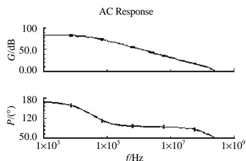
Fig.3 AC response of the amplifier
