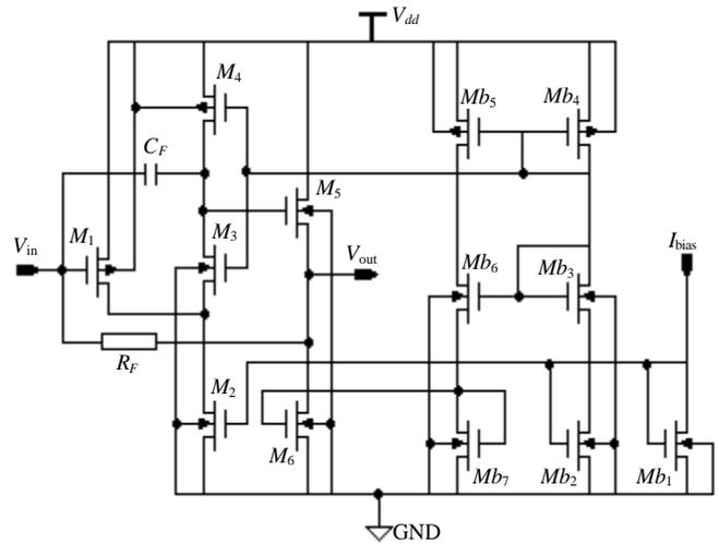
Fig.1 Topology of the charge amplifier
