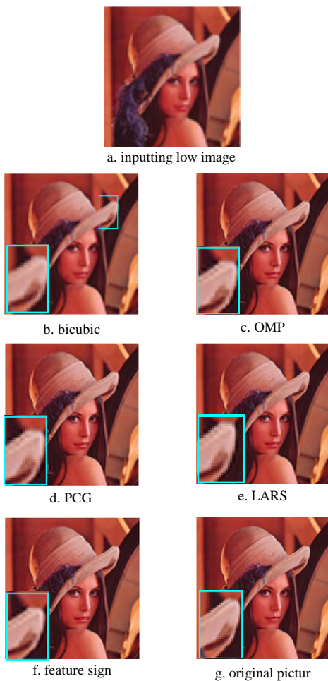
Fig.1 Reconstructed HR images (scaling factor 3) of Lena and the magnified brim of the hat by different methods.
