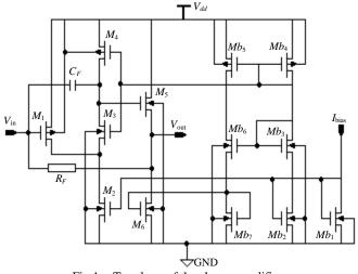
Fig.1 Topology of the charge amplifier
