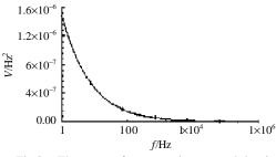
Fig.2 The curve of output noise spectral density
