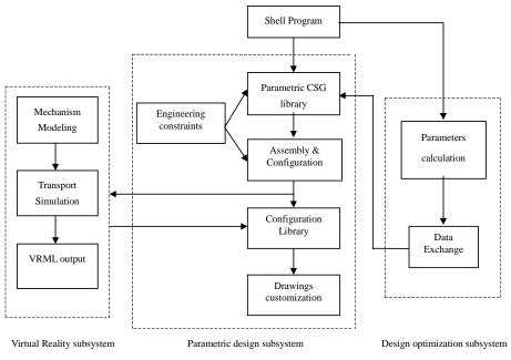
Fig.1 Structure of design automation of blending system
