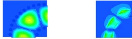
Fig. 3 E-field distribution along SIW and microstrip bends
